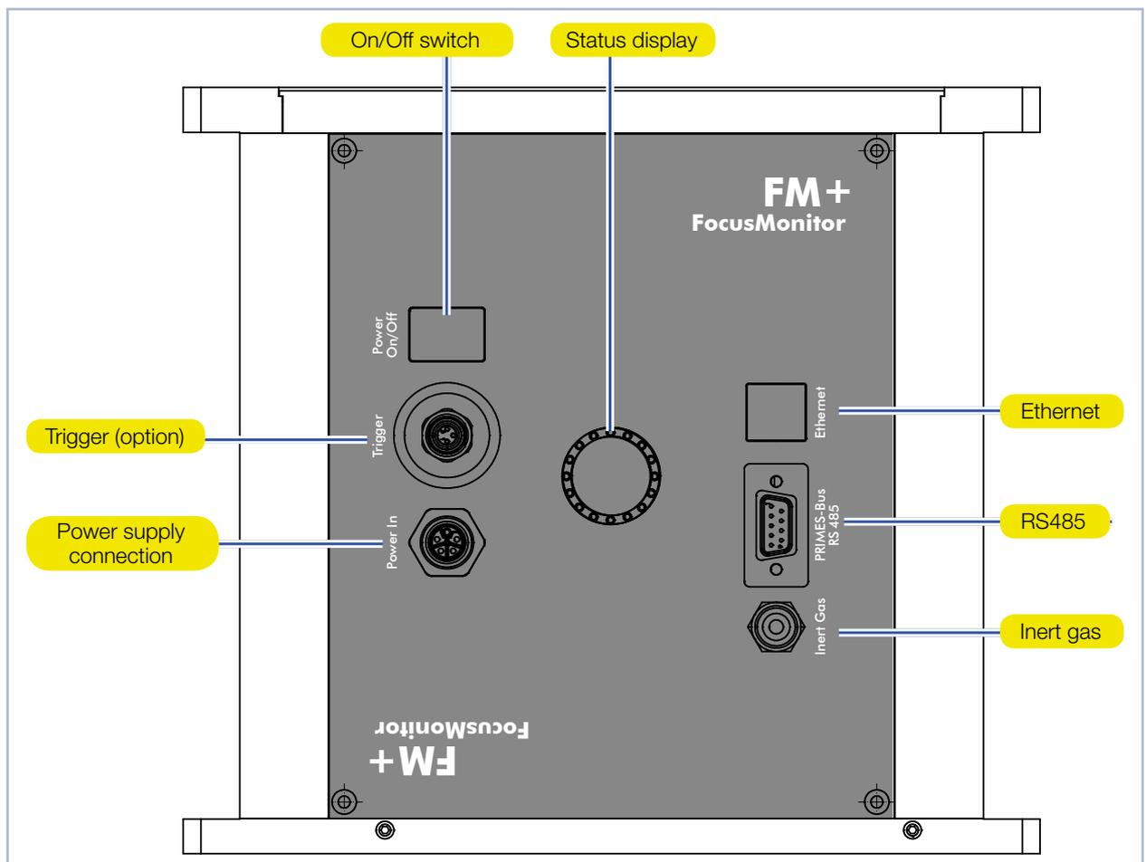
Fig. 8.1: FocusMonitor FM+ connections
