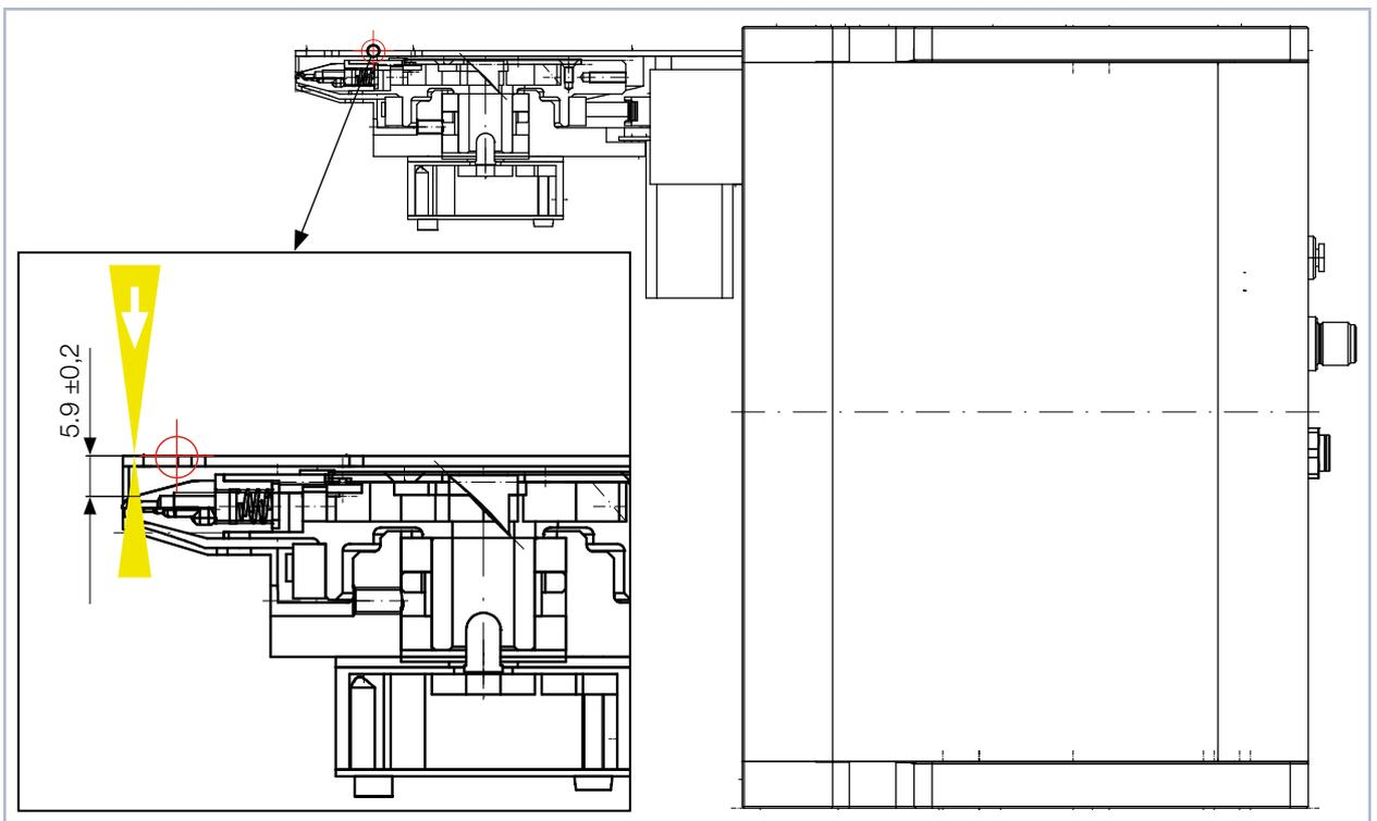
Fig. 11.2: Distance from the aperture in the measuring tip (pinhole) to the reference plane on the bottom of the horizontal carrier
