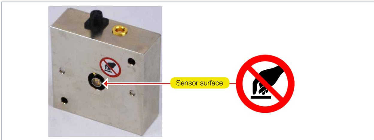
Fig. 18.5: Sensor surface on the detector
