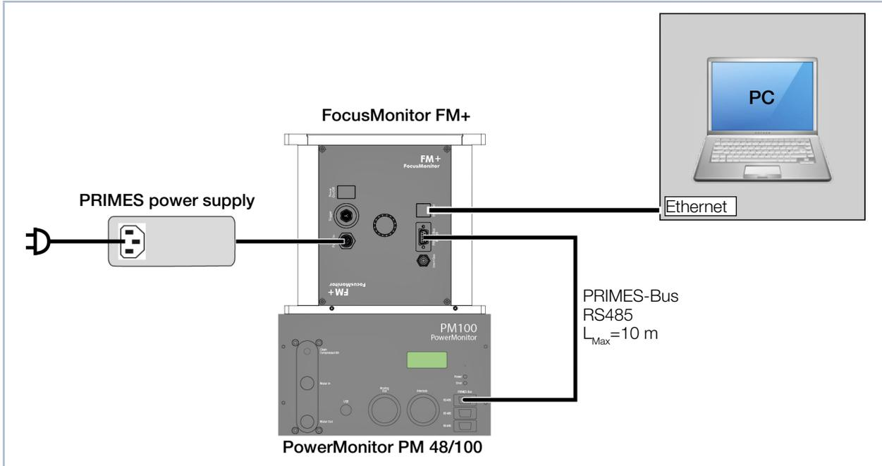
Fig. 8.3: Connection of the FocusMonitor FM+ and PowerMonitor PM 48/100 to the PC
