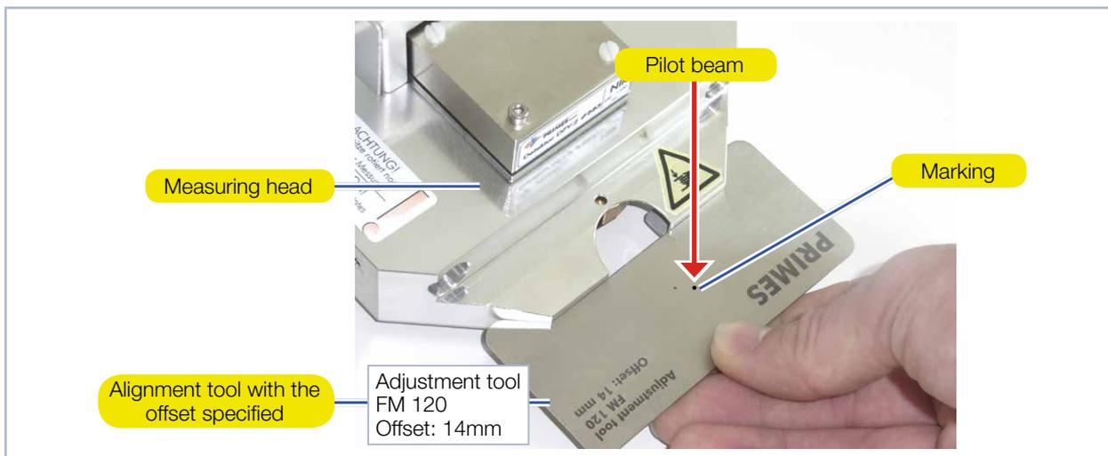
Fig. 7.7: Alignment tool at the measuring head of FocusMonitor FM+
