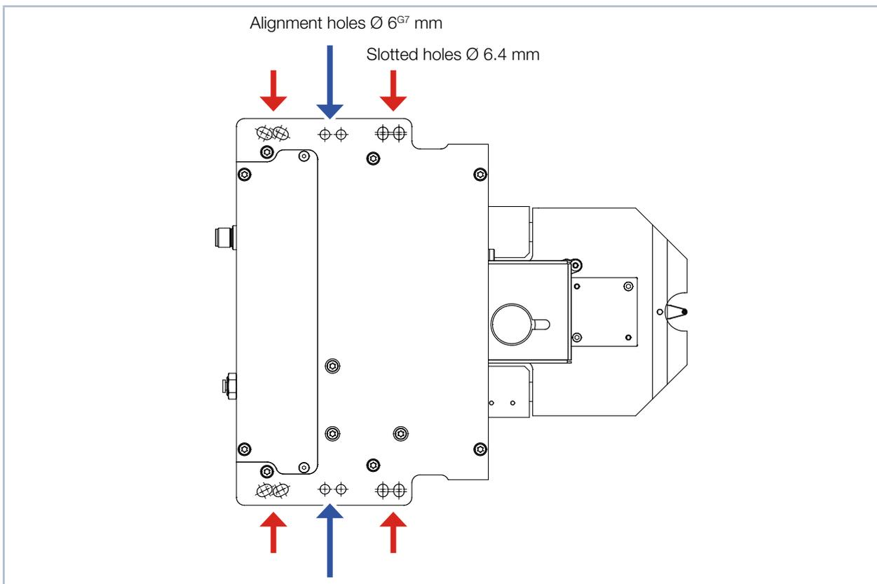
Fig. 7.9: Mounting holes, view from above (same hole pattern below)
