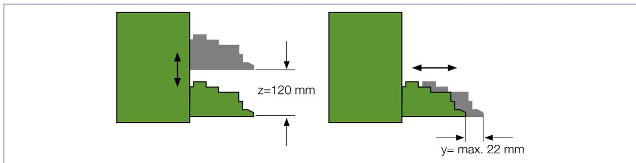
Fig. 7.3: Movement range of the measuring head
