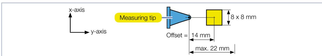
Fig. 7.8: Offset of a measurement window size of 8 x 8 mm
