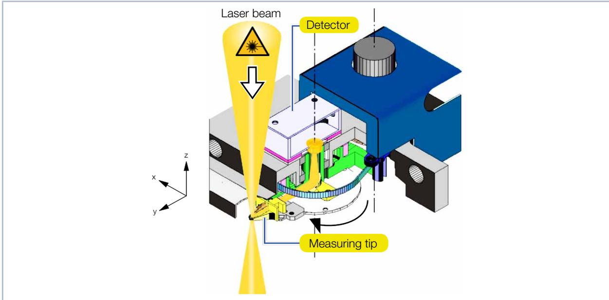
Fig. 5.2: Optomechanical design of the FocusMonitor FM+
