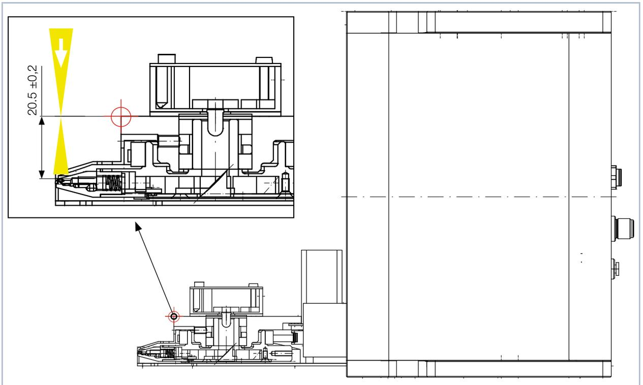
Fig. 11.1: Distance from the aperture in the measuring tip (pinhole) to the reference plane of the horizontal carrier
