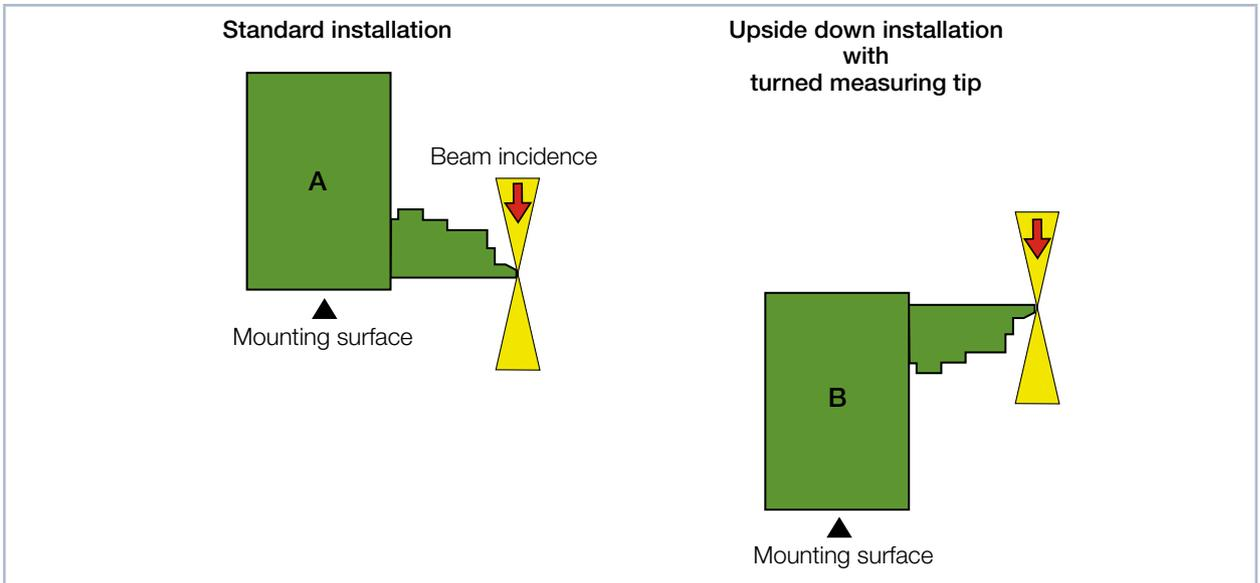
Fig. 7.4: Mounting options for the FocusMonitor FM+
