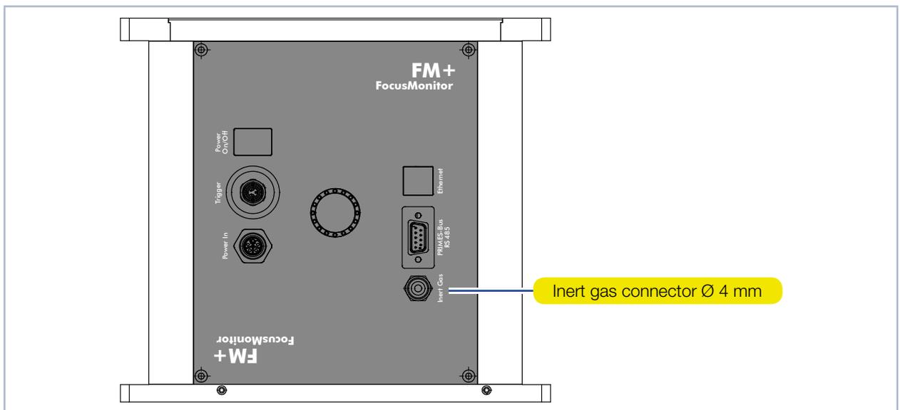
Fig. 9.1: Inert gas connection on the FocusMonitor FM+
