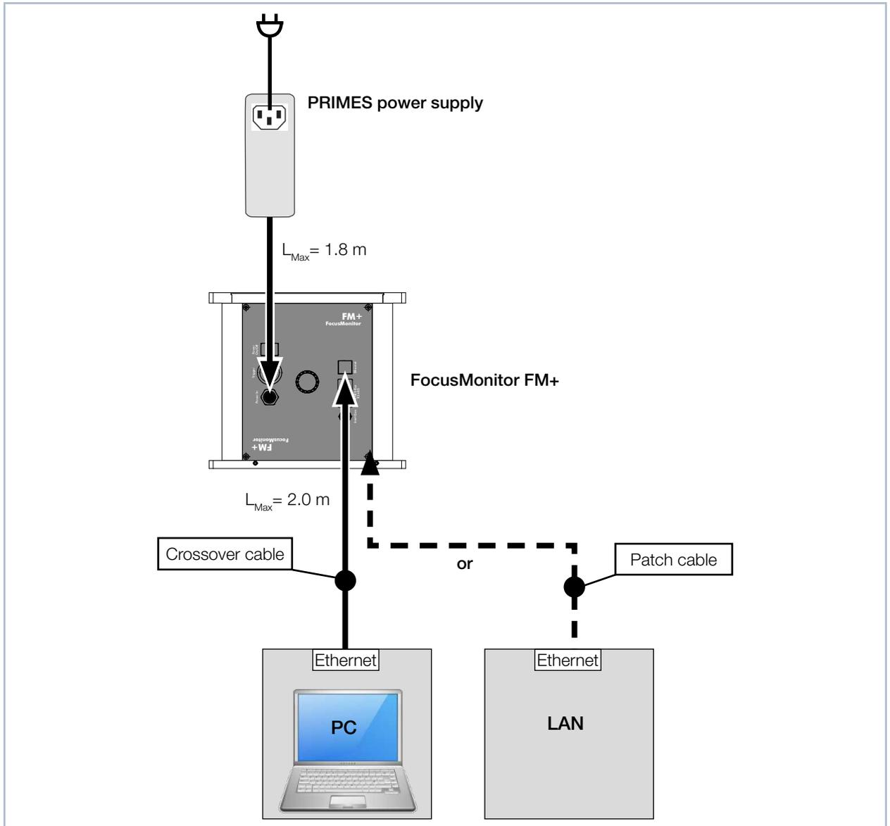
Fig. 8.2: Connection of FocusMonitor FM+
